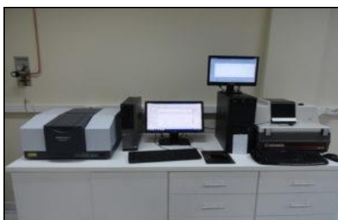
Fig 4: (FTIR). Shimadzu®: IRAffinity 1.
