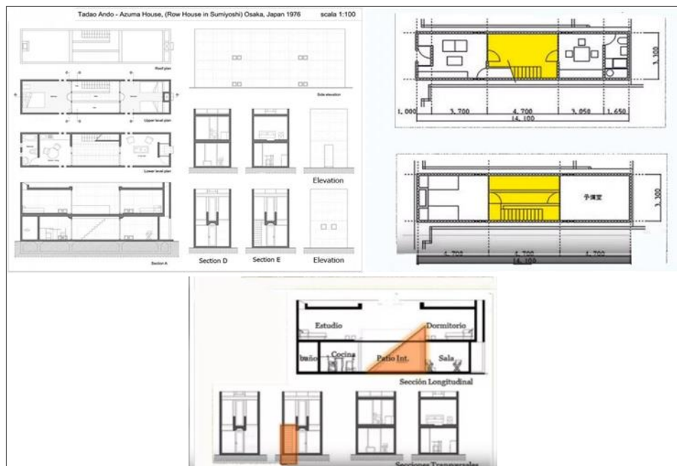
Fig 23, 24 and 25: Azuma house, plan, section and elevation, Azuma house, here we can see that yellow solid color indicates the patio space which brings in more natural light and gives that openness in the house.
