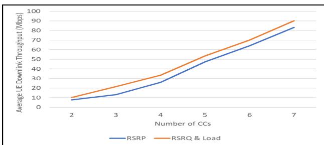
Fig 9: Impact of CCs number to throughput for 20MHz bandwidth and 8MB file size (case b).
