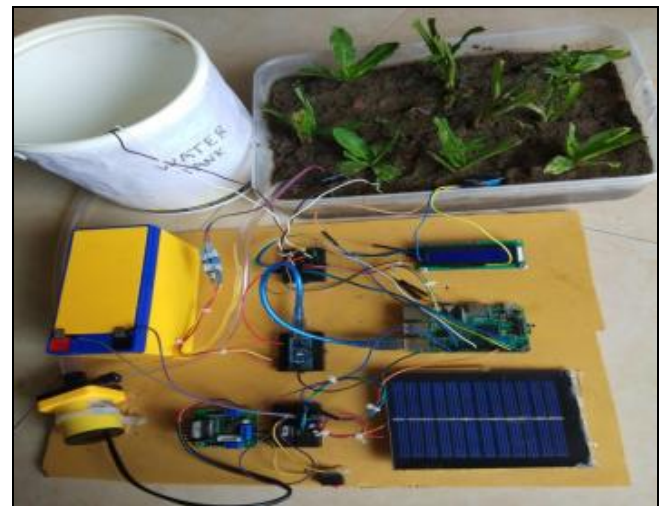
Fig 5: Experimental Setup of IOT Based WSN for Agriculture Field
