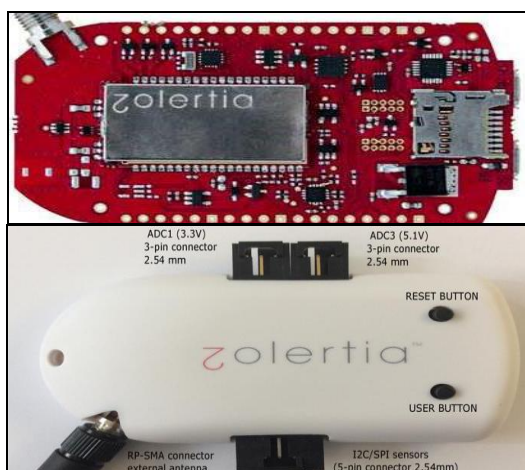
Fig 1: Zolertia Re-Mote and some of its features
